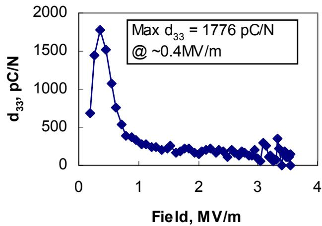
Figure 4. Field dependent  $d_{33}$  obtained by differentiation of the fig. 3 curve.
