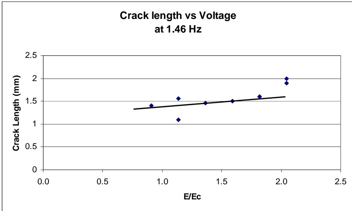
**Fig. 4.** Crack length vs. applied field at a frequency of 1.46 Hz.
