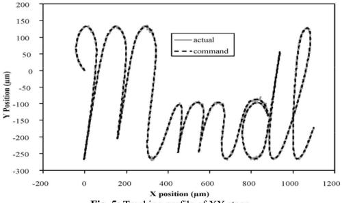
**Fig. 5:** Tracking profile of XY stage.
