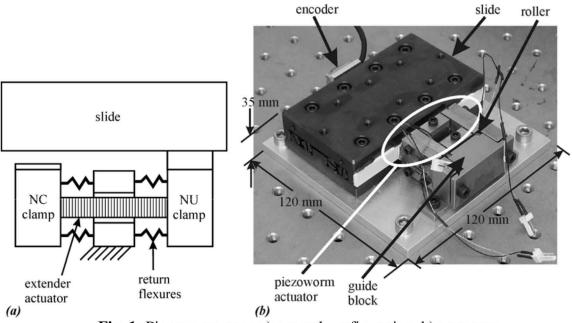
Fig. 1: Piezoworm stage a) general configuration, b) prototype.
