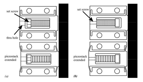
Fig. 2: a) NU clamp operation, b) NC clamp operation.
