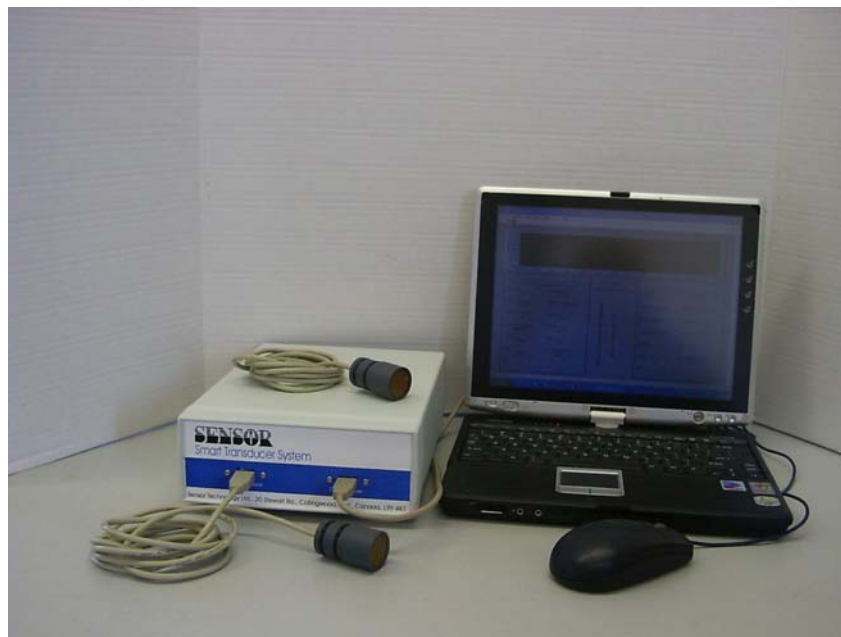
Figure 5: Smart hydrophone system set up
