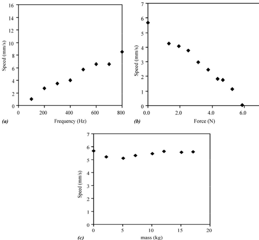
**Fig. 3:** (a)No-load speed versus operating frequency. (b)Speed versus applied force. (c)Speed versus mass.
