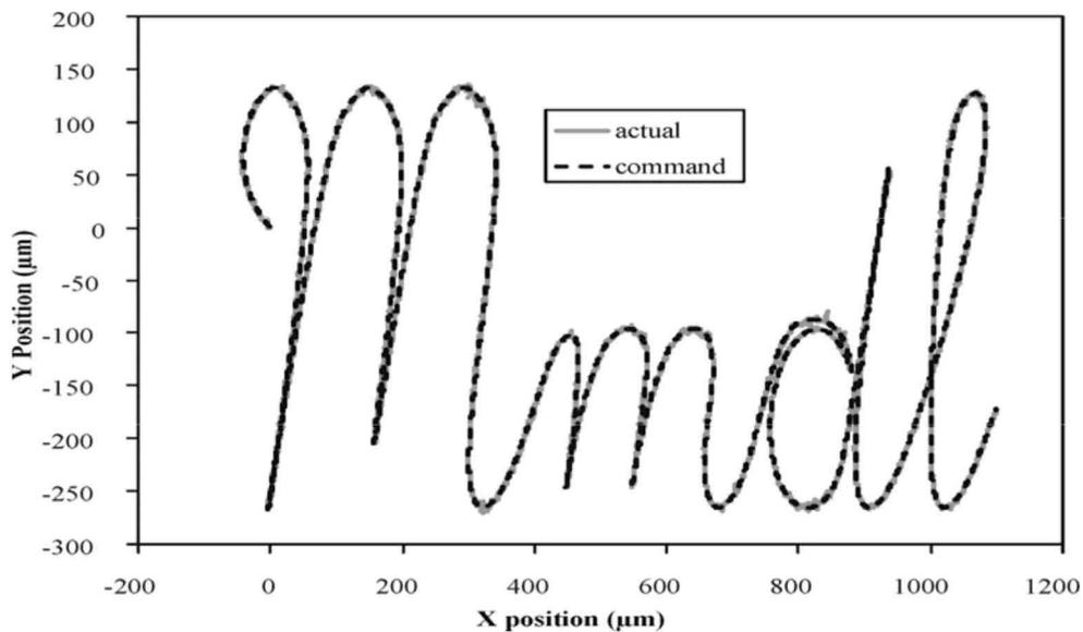
**Fig. 5:** Tracking profile of XY stage.
