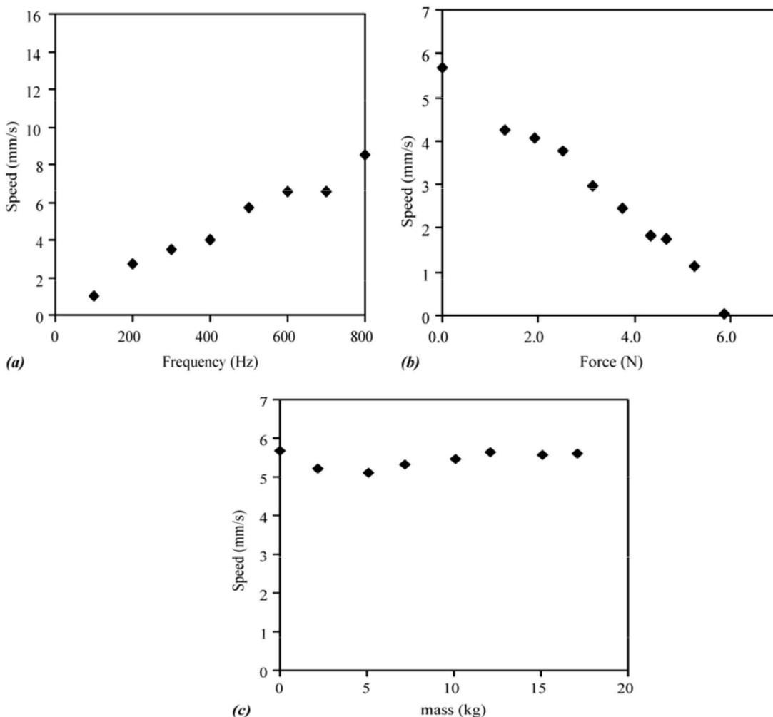
**Fig. 3:** (a)No-load speed versus operating frequency. (b)Speed versus applied force. (c)Speed versus mass.
