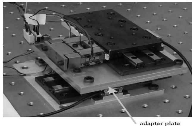
**Fig. 4:** XY stage prototype.
