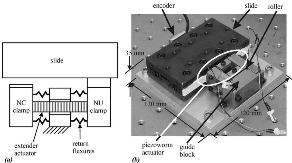
**Fig. 1:** Piezoworm stage a) general configuration, b) prototype.
