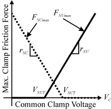
Fig. 5. Clamp friction force capacity vs. voltage characteristic.
