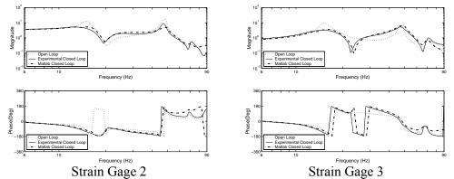
Figure 3: Open Loop and Closed Loop Forced Vibration Frequency Responses of the Smart Fin for Strain Measurement (Controller Input is Strain Gage 2)
