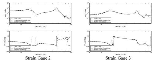
Figure 4: Open Loop and Closed Loop Forced Vibration Frequency Responses of the Smart Fin for Strain Measurement (Controller Input is Strain Gage 3)
