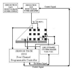
Figure 2: Experimental Setup for Strain Measurement Applications of the Smart Fin
