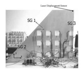
Figure1: The Smart Fin Used in the Study (SG: Strain Gage)
