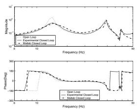
Figure 7: Open Loop and Closed Loop Forced Vibration Frequency Responses of the Smart Fin for Displacement Measurements (Controller Input is Fin Flexural Tip Displacement)
